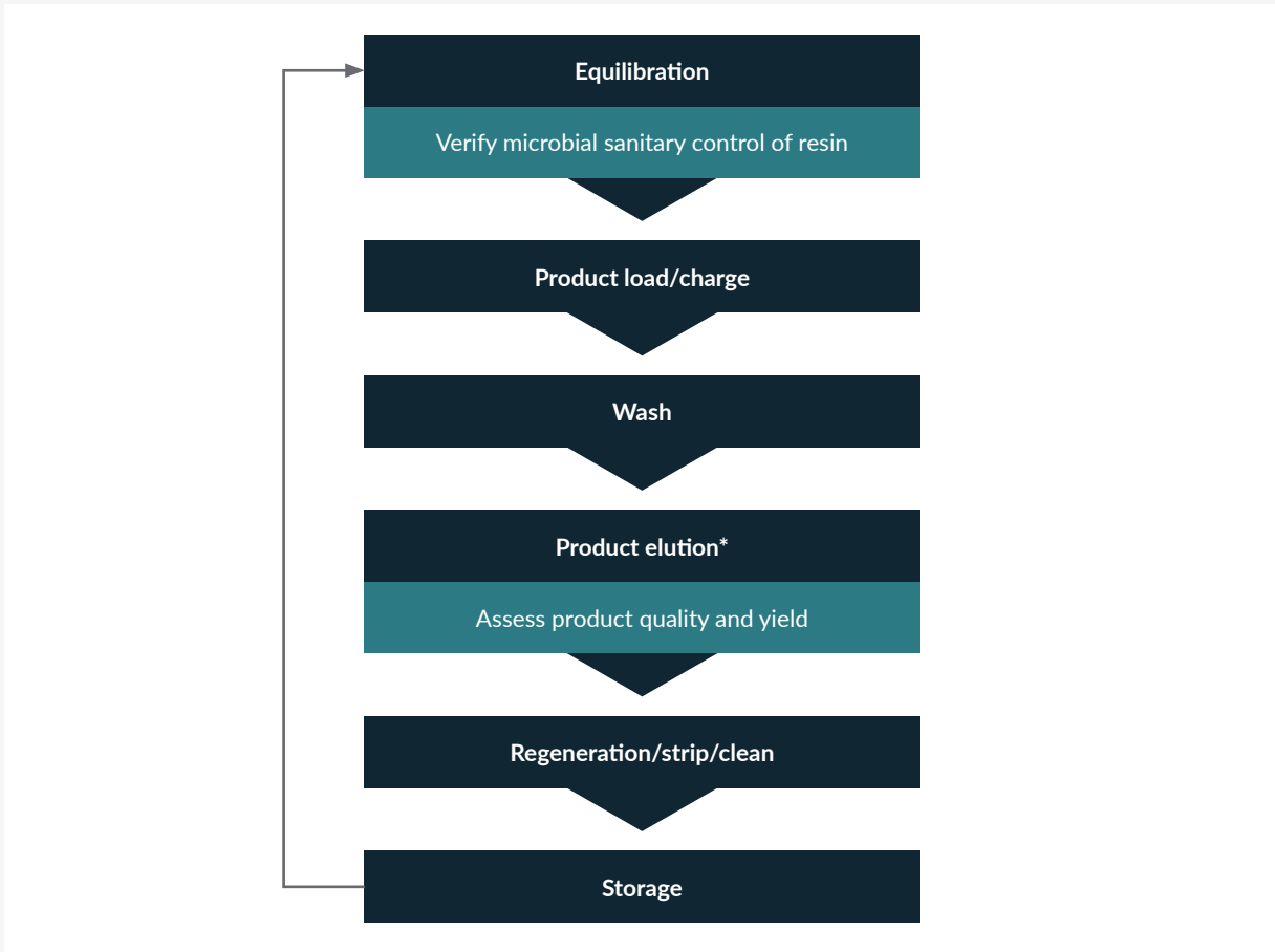
Figure 3: Typical sequence for resin re-use in a single-product process
