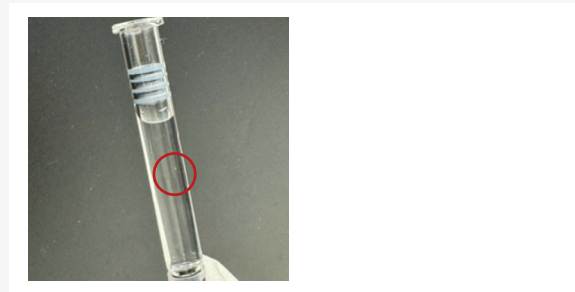
Figure 7: A dummy unit used in conjunction with a vacuum leak detection needle valve
