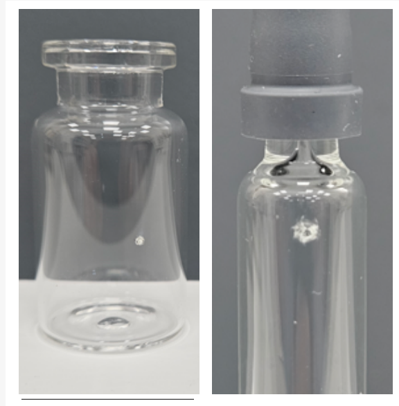
Figure 2: Vial and a syringe both showing a laser-drilled hole
