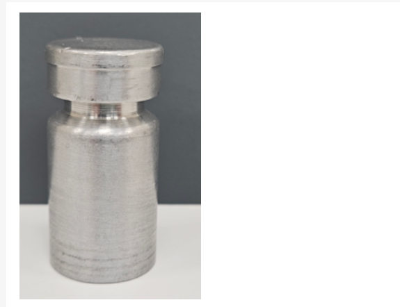
Figure 7: A dummy unit used in conjunction with a vacuum leak detection needle valve
