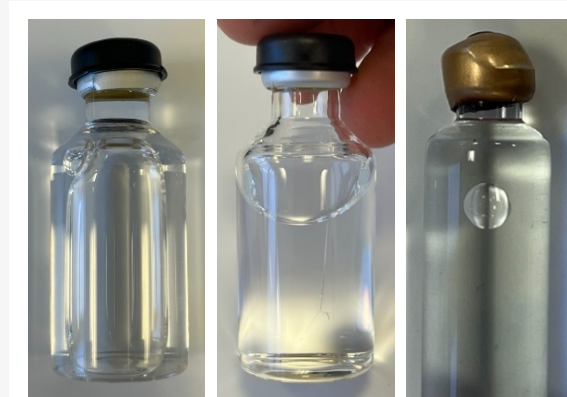
Figure 1: Left, a vial with a crimping defect in the cap. Middle, a vial with a crack in the glass. Right, a cartridge with a deformed cap. Samples with these defects manufactured for CCIT specifically.
